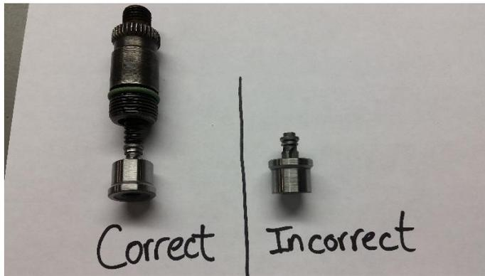
5. Replace and lube the o-ring seals on the threaded portion of the delivery valve holders engine oil, WD-40 or similar.
