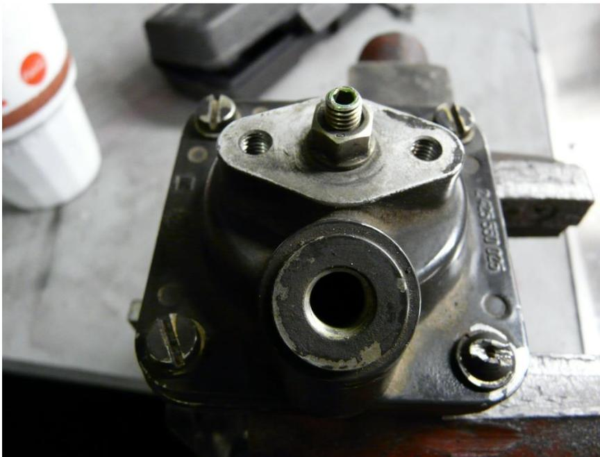
flat-standard screws and grinding a slot in (1) tamper-proof screw and then removing screw. Also grind a slot in the tamper-proof screw on the small pre-boost fuel cover and remove the cover. A sharp chisel can also be used to make a slot. Pliers or vice grips are another method for tamper screw removal.
