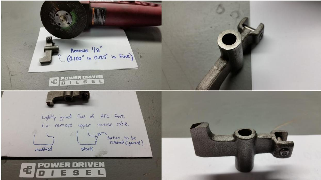
8. Using a grinder or cut-off wheel, remove 1/8" (0.125") from the guide barrel of the AFC foot, for maximum AFC foot travel a minimum 0.100" must be removed. Optional: lightly grind the face of the AFC foot to remove the reverse/negative rake on the upper portion of the foot. The dark portion of the foot face in the picture is left stock, only the upper half is lightly ground flat to remove the upper reverse rake.
