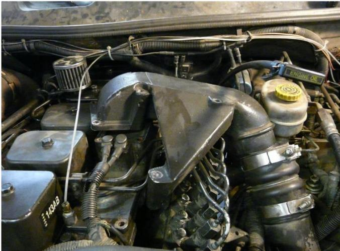
1. Remove air-intake horn by removing (5) 10mm bolts, (1) 10mm dipstick bolt, and loosening (1) 7/16" t-bolt clamp on the air-take hose. Take care when removing the intake horn to not damage the gasket at the mating surface, normally this gasket can be reused, but if it is damaged a replacement is available from Cummins, part number 3913352.
