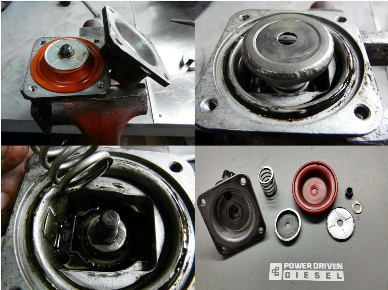
6. Under the AFC back cover is a red rubber-like diaphragm. Remove the 10mm nut, small washer, large washer, diaphragm, inner cupped washer, and stock AFC spring.
