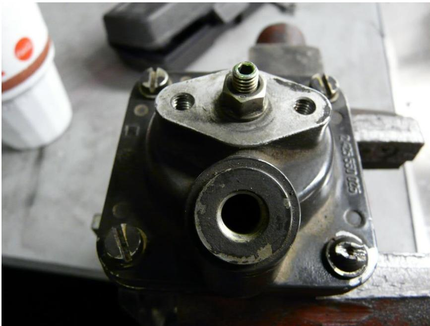
flat-standard screws and grinding a slot in (1) tamper-proof screw and then removing screw. Also grind a slot in the tamper-proof screw on the small pre-boost fuel cover and remove the cover. A sharp chisel can also be used to make a slot. Pliers or vice grips are another method for tamper screw removal.
