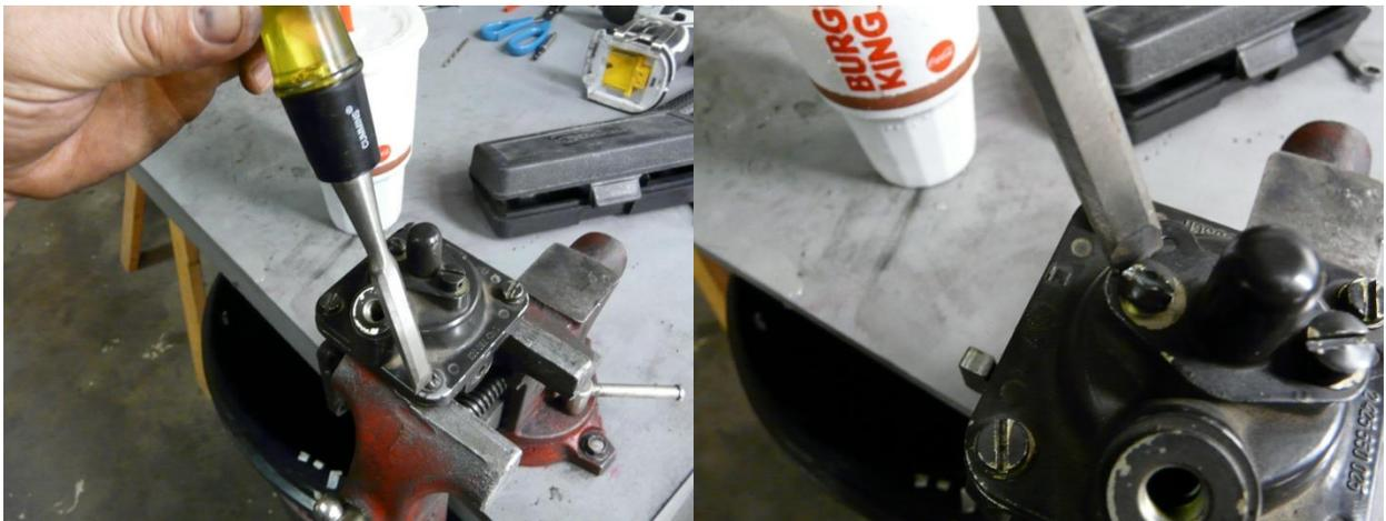
5. Take the AFC to a suitable working location (work bench). Remove AFC cover by removing (3)
